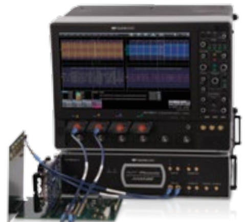
PCIe Gen3 Link Equalization testing using the SDA8Zi-A and the PeRT 3 Phoenix.
